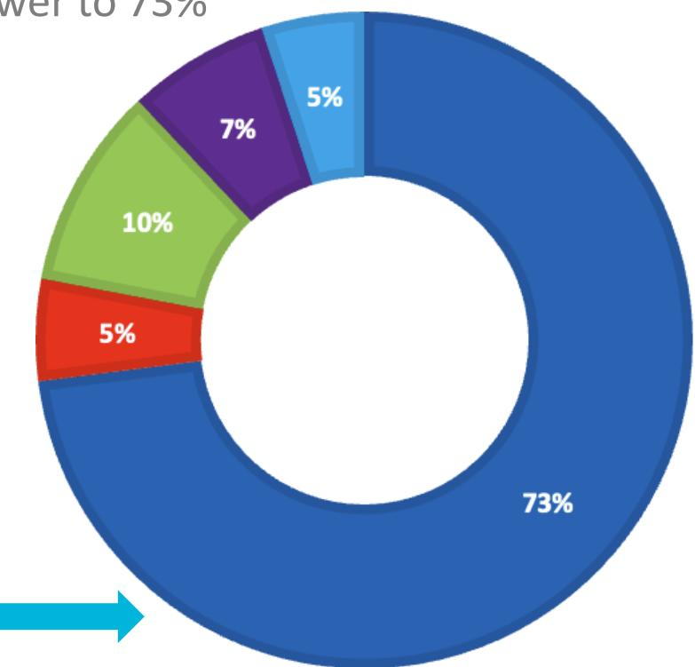
When moving to direct-to-chip liquid cooling, computing moves from 40% to 73%
