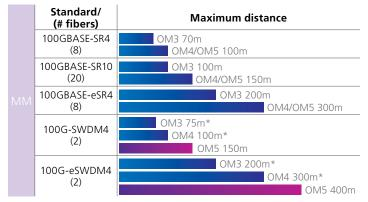
Figure 6: Short reach 100G applications in the data center \* OM3/OM4 effective modal bandwidth only specified at 850nm
