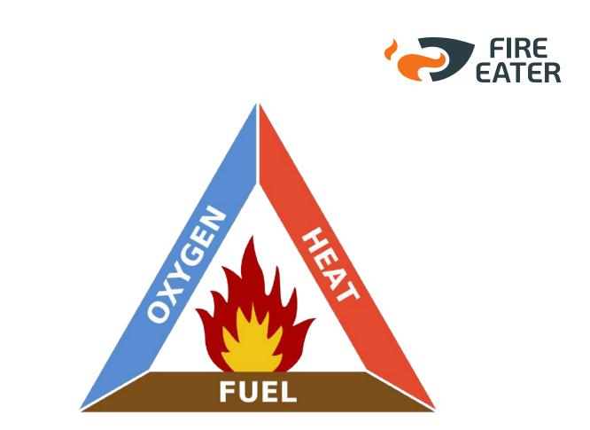
**Inergen** extinguishes a fire by blending a mixture of natural gases into the room, thus lowering the oxygen level from 20.9 % to approx. 12 % that suffocates the fire with a good safety margin.
