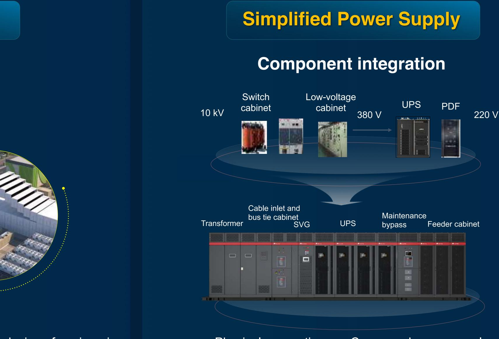
Physical connections → Converged power supply
