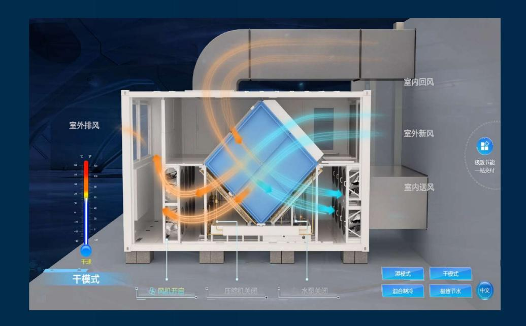
Maximized use of free cooling sources and one heat exchange
