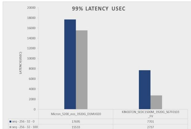
Figure b) Sequential BW(MB/s) read/write and latency(usec) comparison of DC1500M 1920G and Micron 5200 ECO 1920G SATA SSD. Tested on a single physical drive attached as a secondary to a Linux system with foo v3.17 once the SSDs have reached a steady state of performance. Based on a block size of 256k and a queue depth of 32
