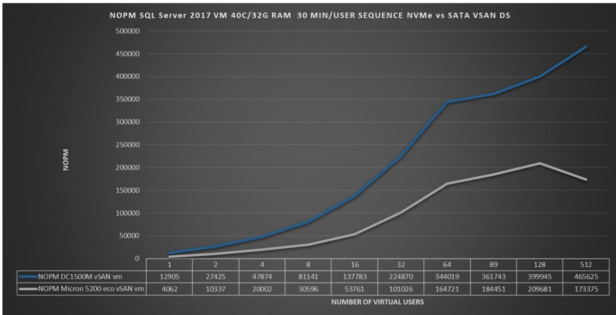
Figure 4.3 Test 3 TPM comparison SQL Server 2017 DB stress test on Micron 5200 eco SATA and DC1500M NVMe SSD vSAN datastore
