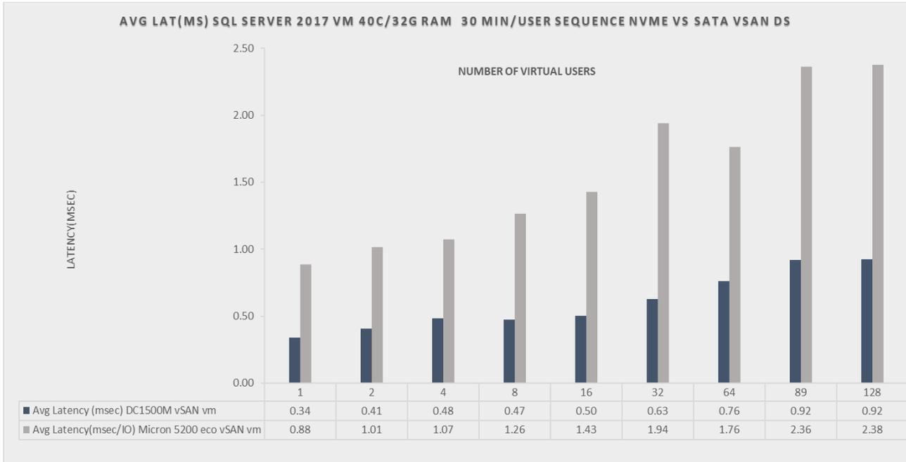
Figure 4.4 Test 3 avg latency(ms) comparison SQL Server 2017 DB stress test on Micron 5200 eco SATA and DC1500M NVMe SSD vSAN datastore
