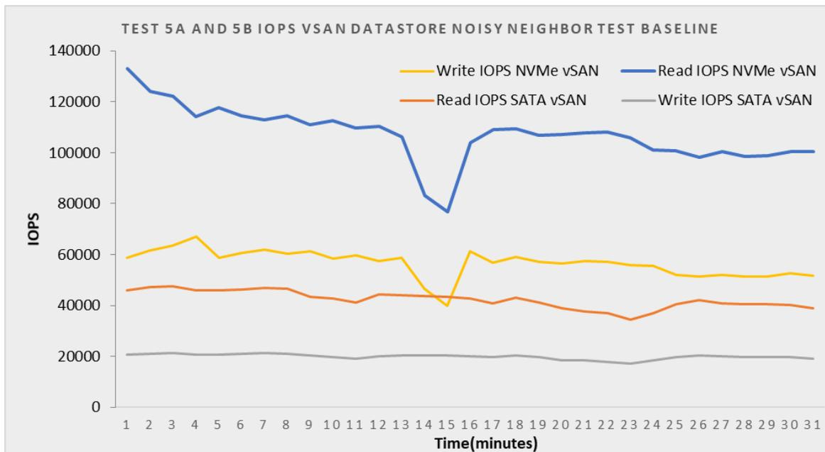
Figure 6.4 Test 5a and 5b Noisy neighbour IOPS, DC1500M NVMe and Micron 5200 eco vSAN datastore
