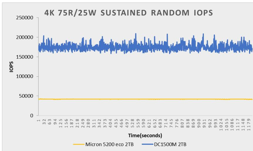
Figure a) Second-by-second IOPS comparison of DC1500M 1920G and Micron 5200 ECO 1920G SATA SSD. Tested on a single physical drive attached as a secondary to a Linux system with foo v3.17 once the SSDs have reached a steady state of performance. Based on a block size of 4k, read percentage of 75% and a queue depth of 32
