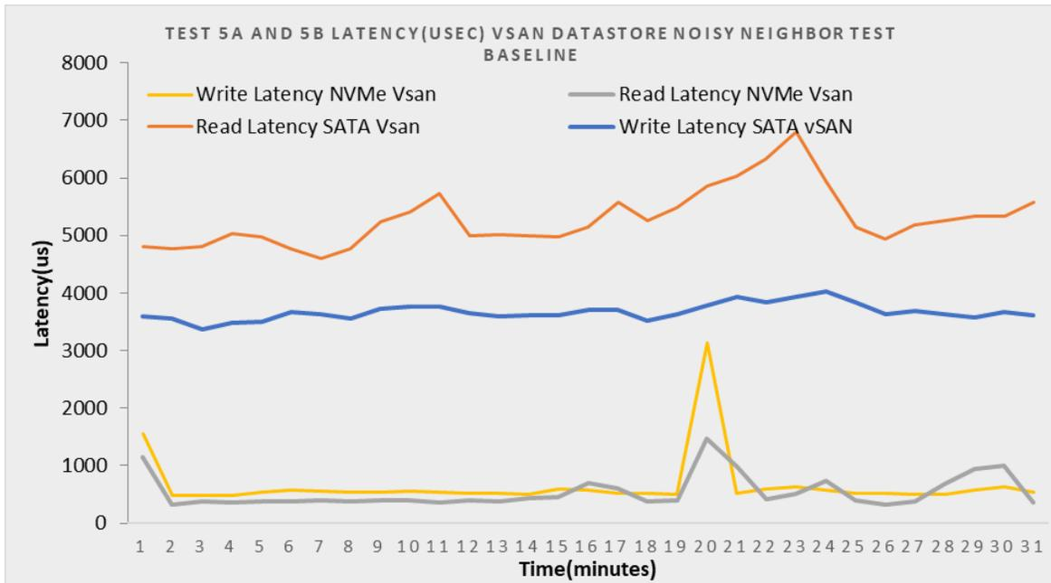
Figure 6.5 Test 5a and 5b Noisy neighbour latency, DC1500M NVMe and Micron 5200 eco vSAN datastore
