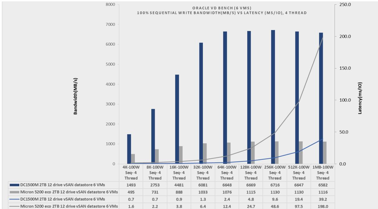
Figure 1.5 DC1500M vSAN datastore vs Micron 5200 eco vSAN datastore, 100W/OR, sequential, QD=8, threads=4, HCBench 6 VMs read throughput(MB/s) and average read latency(ms/IO)
