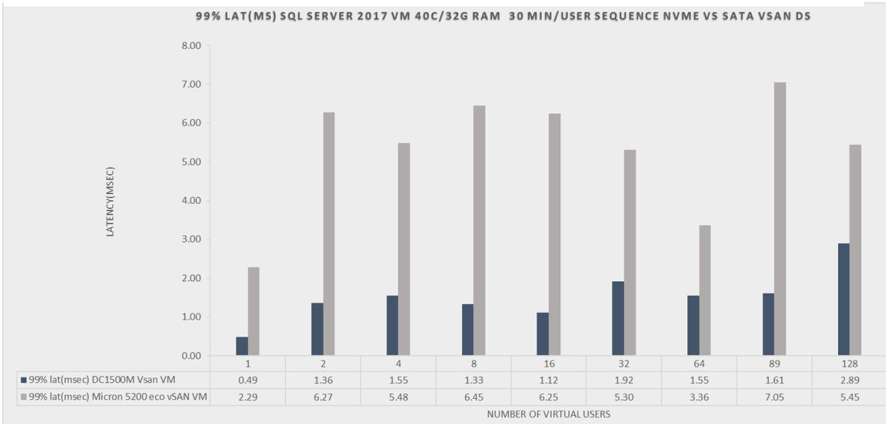
Figure 4.5 Test 3 99<sup>th</sup> % latency(ms) comparison SQL Server 2017 DB stress test on Micron 5200 eco SATA and DC1500M NVMe SSD vSAN datastore
