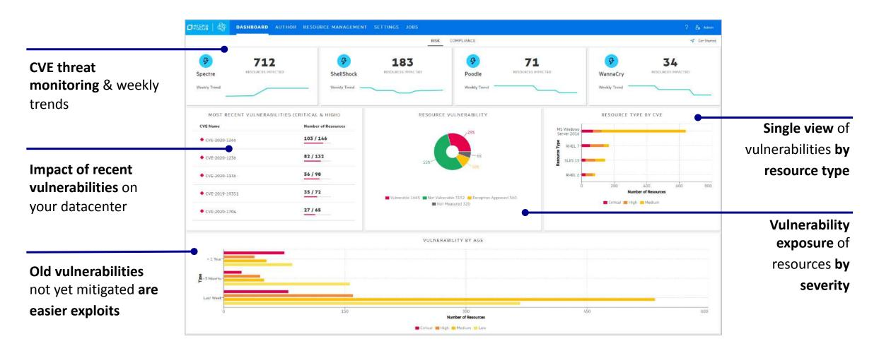
The DCA Risk Dashboard uses **National Vulnerability Database** (NVD) data, patch metadata and patch scan data to identify vulnerabilities in the datacenter
