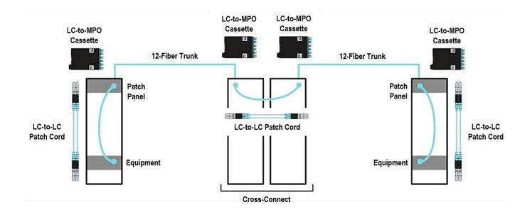
Figure 4. Cross-connect plant model.
