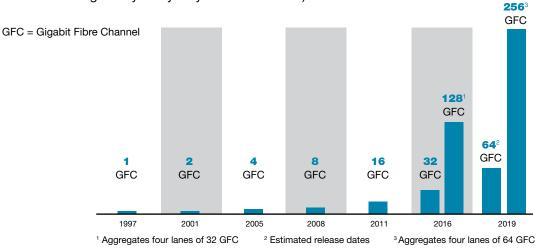
Figure 1. Fibre Channel development since 1997.
