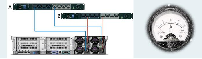
Professionally planned environments therefore rely on components with an N+1 power supply<sup>2</sup>. The devices are connected to different phases and power strips, which in turn are connected to different circuits.
