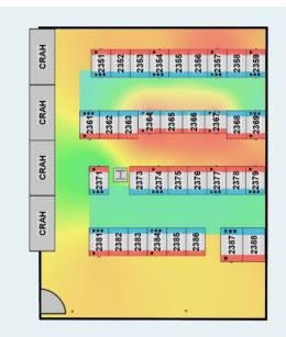
Example of a granular temperature measurement with clear recognizable temperature problems inside and outside the cold aisle containment due to missing seals, incorrect installations and narrow aisle widths.
