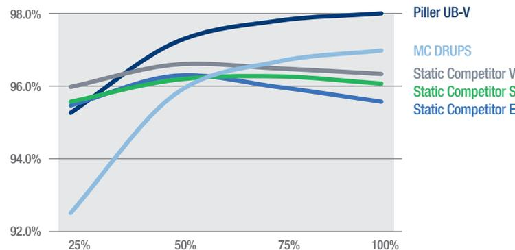
Efficiency comparison of battery-backed electrically coupled UPS types and mechanically coupled UPS in on-line mode.
