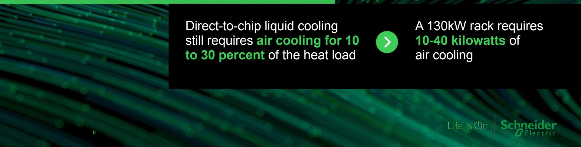
Direct-to-chip liquid cooling still requires **air cooling for 10 to 30 percent** of the heat load
