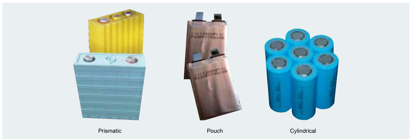
Fig. 3 - Different Li-Ion cell designs.
