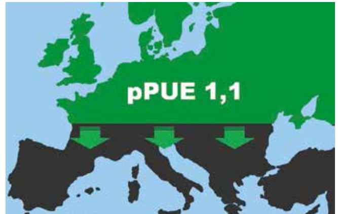
Figure 2. Adiabatic cooling allows for pPUE values as low as 1.1 even in southern EMEA countries.
